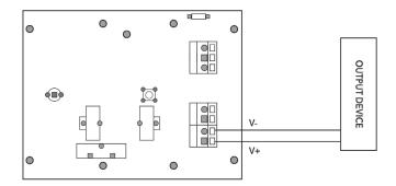
Wiring example for the relay switch output.
