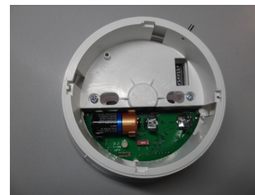
Picture 5 - secondary battery inserted
