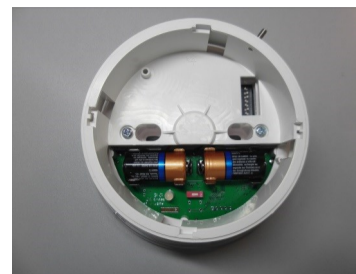
Picture 6 - primary and secondary batteries inserted
