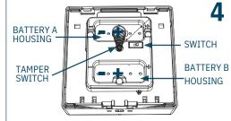
Ensure the programming switch on the MCP is in position ON.
