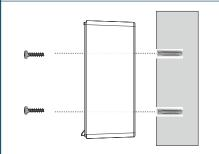
Screw the back box to the wall using all fixing holes and the supplied screws.
