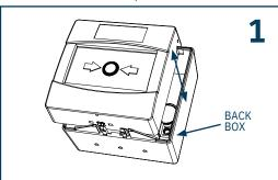
Remove the MCP front from the back box using key provided.
