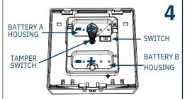
Ensure the programming switch on the MCP is in position ON.
