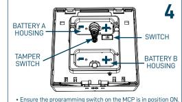
• Fit the 2x CR123A batteries ensuring you have checked they are the correct way round observing the polarity indications.
