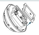
Remove the battery compartment cover on the base on the detector.
