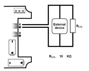
Wiring example for the relay switch output.
