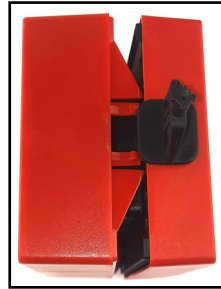
Picture 10 - front device block removal from its wall mounting back box
