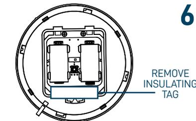
Remove the batteries' insulating tab ensuring the batteries are kept in their lodgement.
