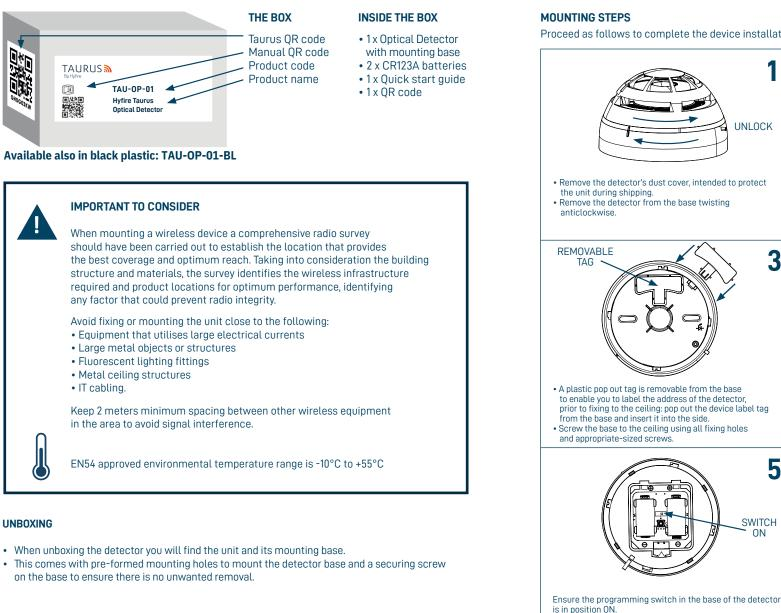
Proceed as follows to complete the device installation.
